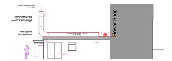
The flue/extract has now been designed to ensure the output pipe is above the existing eaves height of the neighbouring properties and the system now incorporates advanced filtration systems within it to ensure the neighbouring residents and units are not detrimentally affected by any smells or noise. The applicants submitted noise assessment concludes that:
